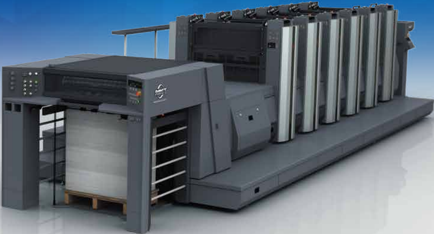
790ST-5+CC+SLD (5-color straight press with coating unit, semi-long delivery model)
