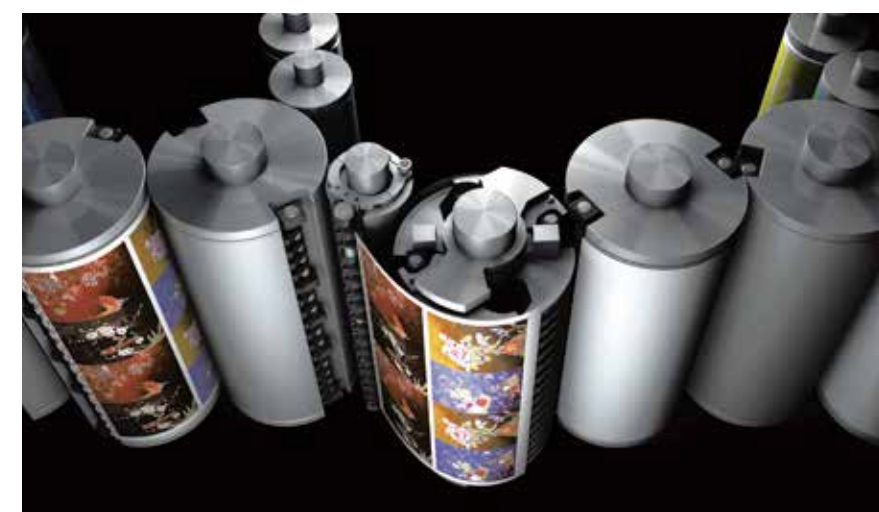
Double/double/single-diameter cylinder perfecting mechanism*
