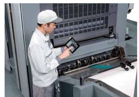
Remote monitoring of Press Information Display by Tablet PC
