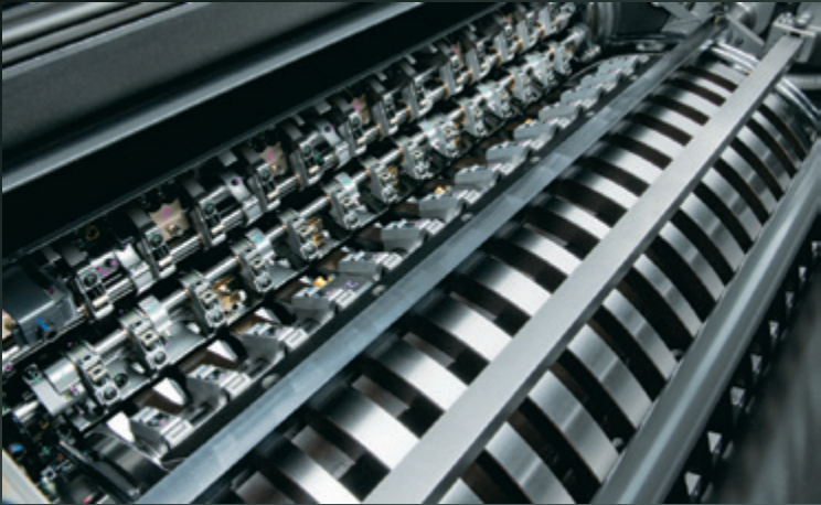
'Double – Double – Single' Perfecting Cylinder configuration Compared to a 'single – double – single' design, this new cylinder configuration ensures stable sheet transport and high-performance perfecting that reduce the possibility of scratches and marking.
