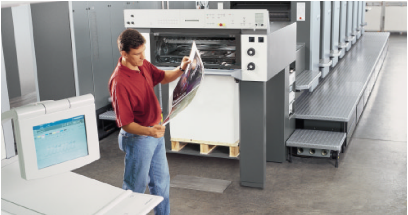
The venturi sheet guide plates carry the sheets onto the delivery pile on an air cushion, without any marking.
